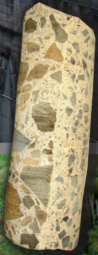
A core sample made from the dam concrete mixed with the 'new' concrete of the panel executed.
